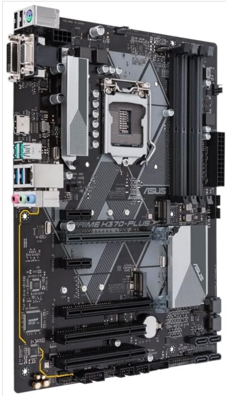
Figure 3: Angled view of the motherboard, showing the location of the dual M.2 slots and PCIe expansion slots.
