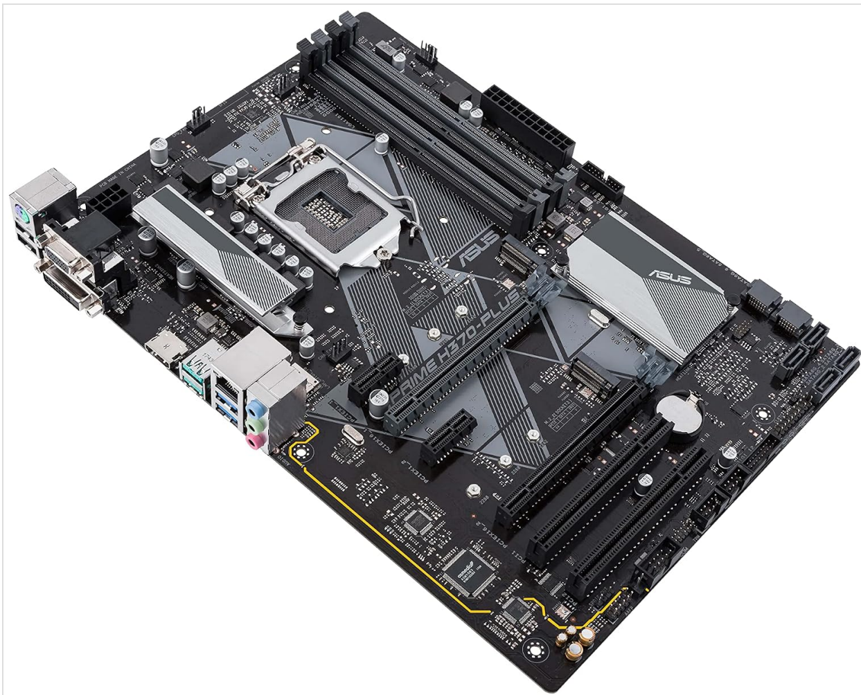
Figure 1: Top-down view of the ASUS Prime H370M-Plus motherboard. This image displays the central LGA1151 CPU socket, four DDR4 RAM slots, multiple PCIe slots, dual M.2 slots, and various I/O ports and headers.
