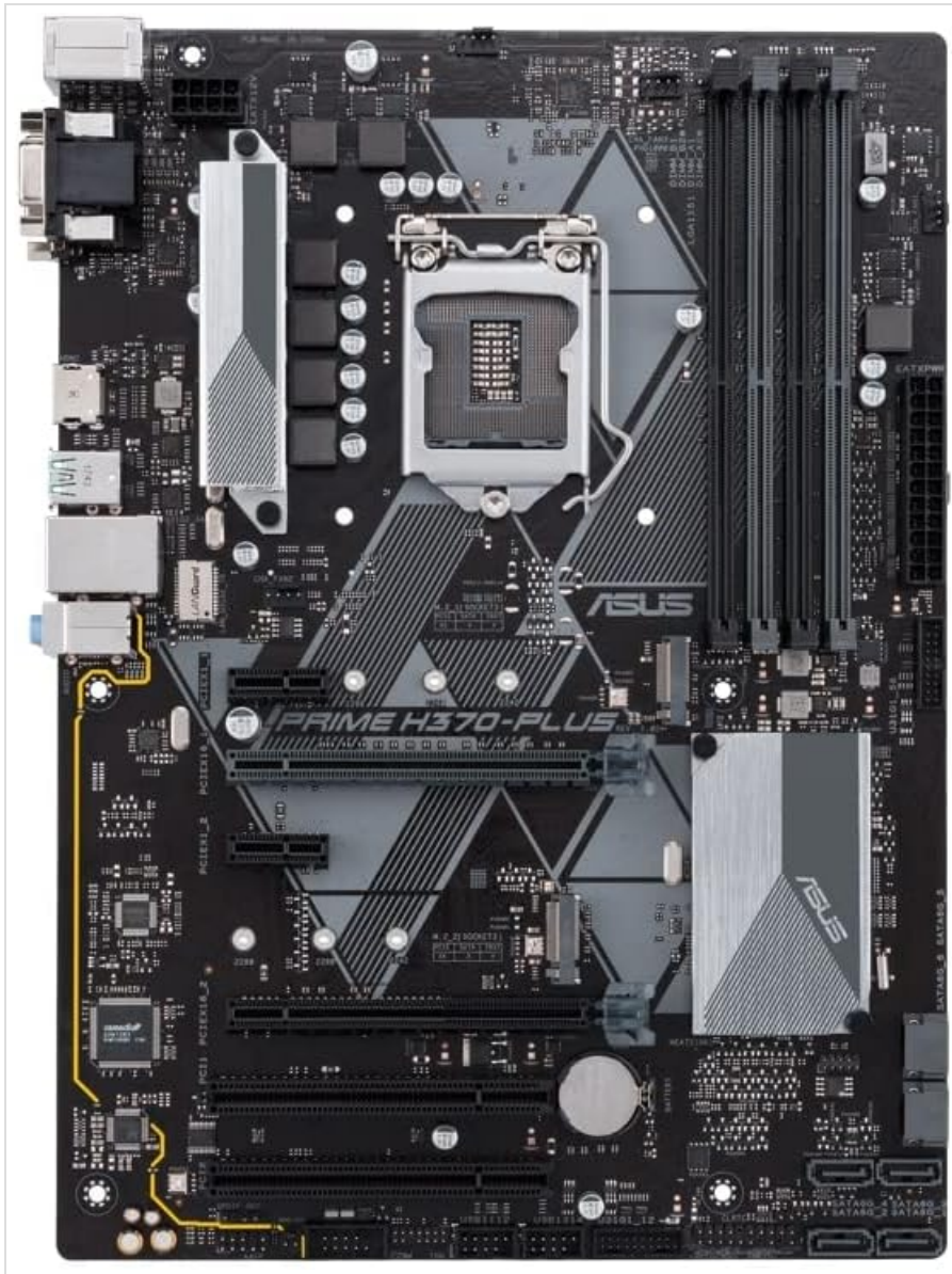
Figure 2: Close-up view of the LGA1151 CPU socket. Note the orientation key (triangle) for correct CPU placement.
