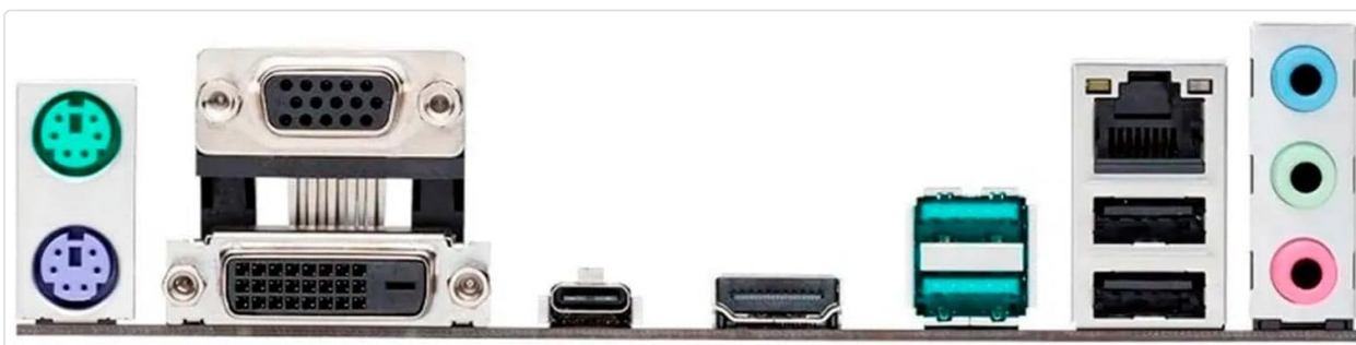
Figure 2.4: Close-up of the rear I/O panel, displaying the various ports including USB, HDMI, DVI, VGA, LAN, and audio jacks.
