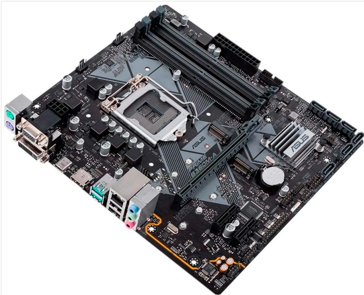
Figure 2.3: An angled perspective of the motherboard, providing a clearer view of the PCIe slots, SATA ports, and the chipset heatsink.
