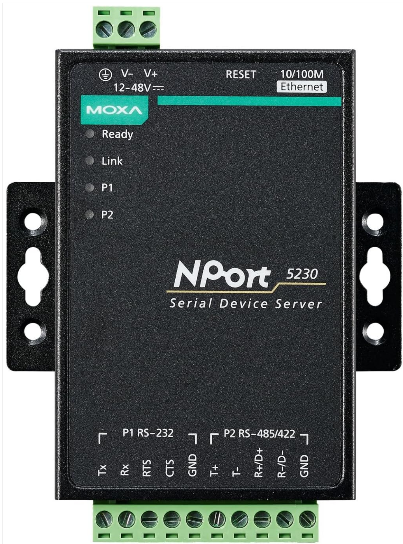
Figure 1: Front view of the MOXA NPort 5230 Device Server, showing the MOXA logo, LED indicators, Ethernet port, and serial ports (P1 RS-232, P2 RS-485/422) with terminal blocks.
