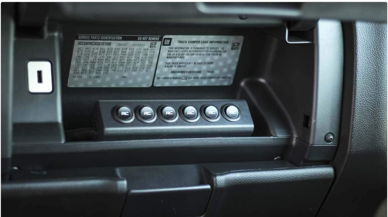
Figure 3.3: The MLC-6 switch panel discreetly mounted in a glove compartment.
