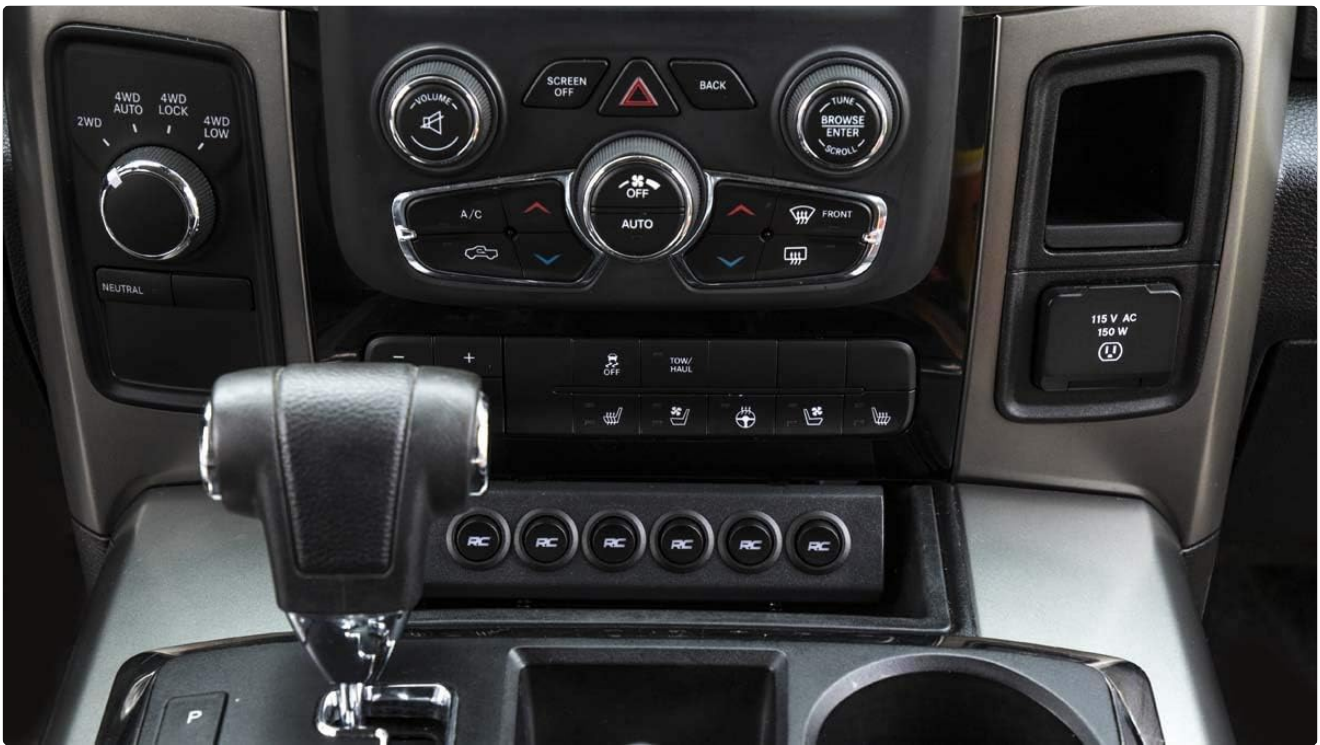
Figure 3.2: Example installation of the MLC-6 switch panel in a vehicle's interior.
