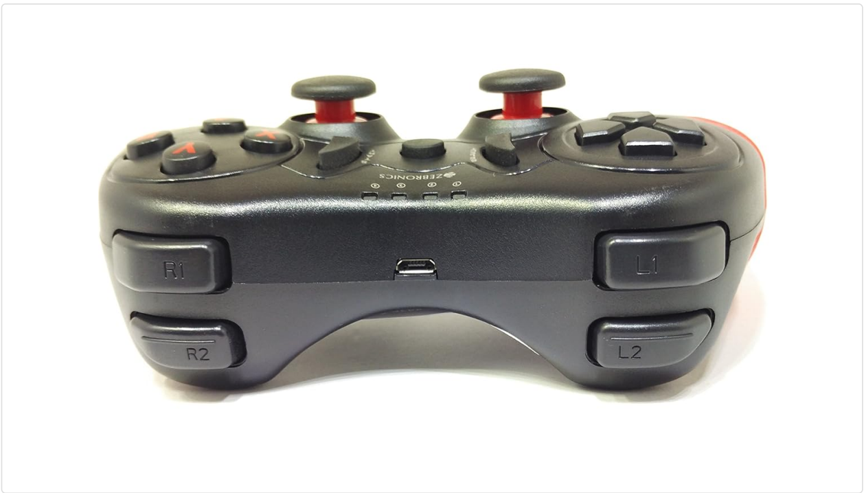
Image 3: Top view of the ZEB-DB250JP gamepad, highlighting the Micro USB charging port located between the L1/R1 and L2/R2 triggers.
