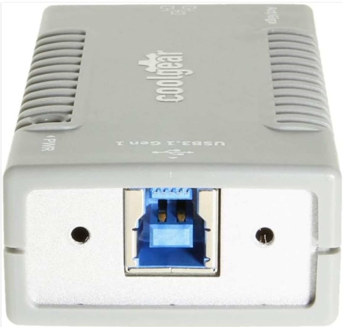
Figure 4.1: USB 3.1 Gen 1 Type-B port for host connection.
