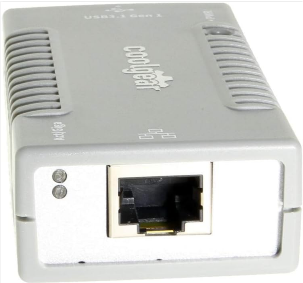
Figure 4.2: RJ45 Gigabit Ethernet port with LINK/ACT and SPEED LEDs.
