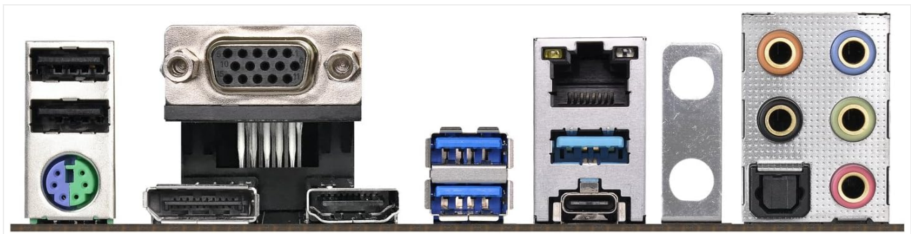
Image: Close-up view of the rear I/O panel, showing various ports including USB, LAN, audio, and video outputs.
