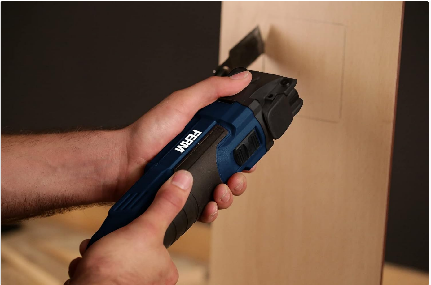
Figure 4: The multi-tool performing a plunge cut into a wooden surface.
