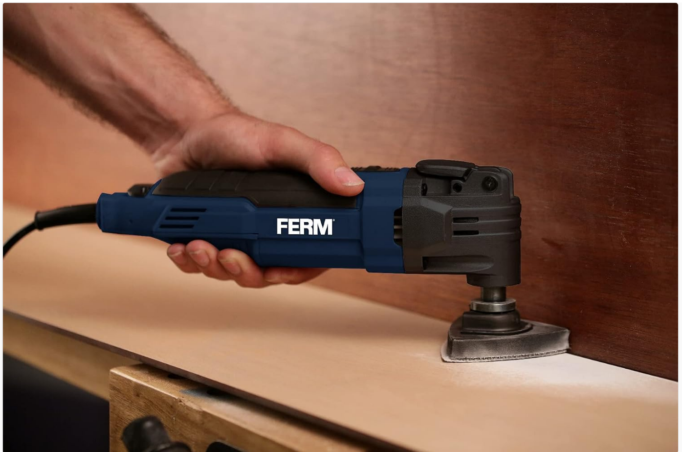
Figure 5: Sanding the edge of a wooden workpiece using the multi-tool with a sanding pad.
