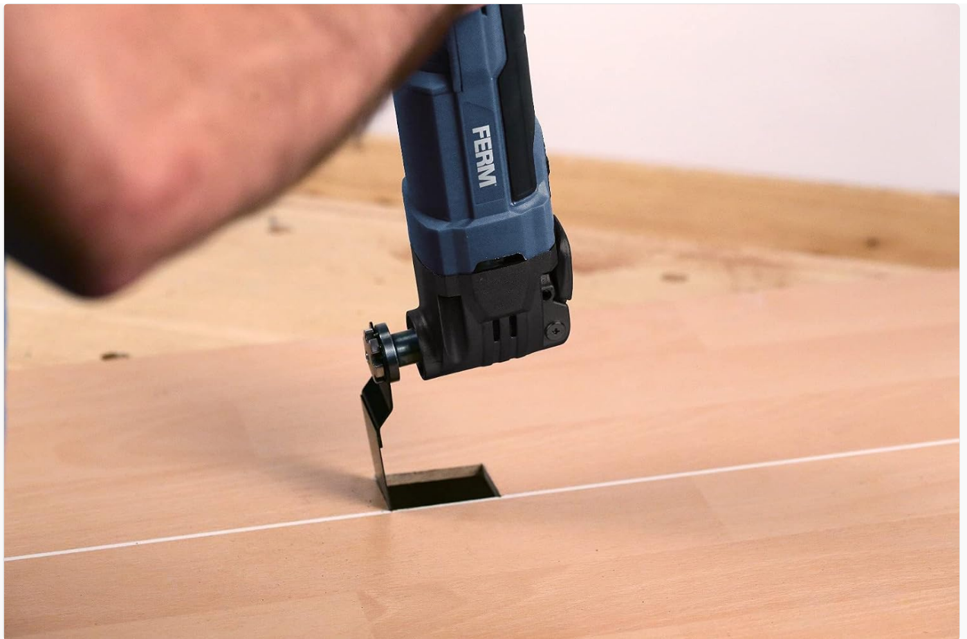
Figure 3: Using the multi-tool with a scrape knife to remove material from a surface.
