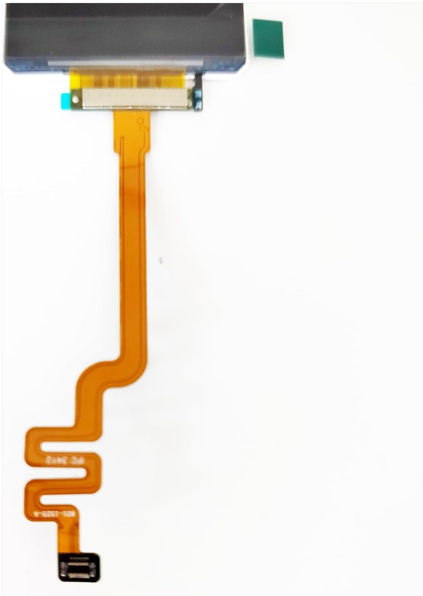
Figure 2: Back view of the LCD Display Screen Replacement, showing the flex cable connection point.
