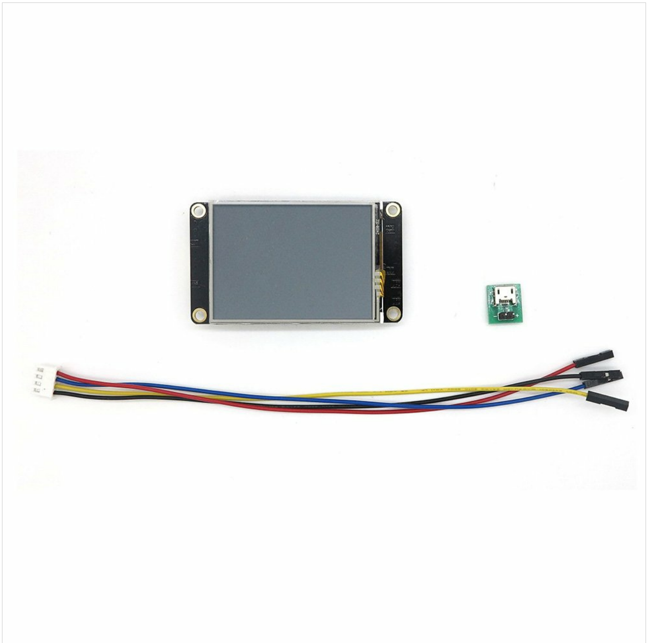
Image 1.1: Front view of the NEXTION Enhanced 4.3 inch NX4827K043 Display.
