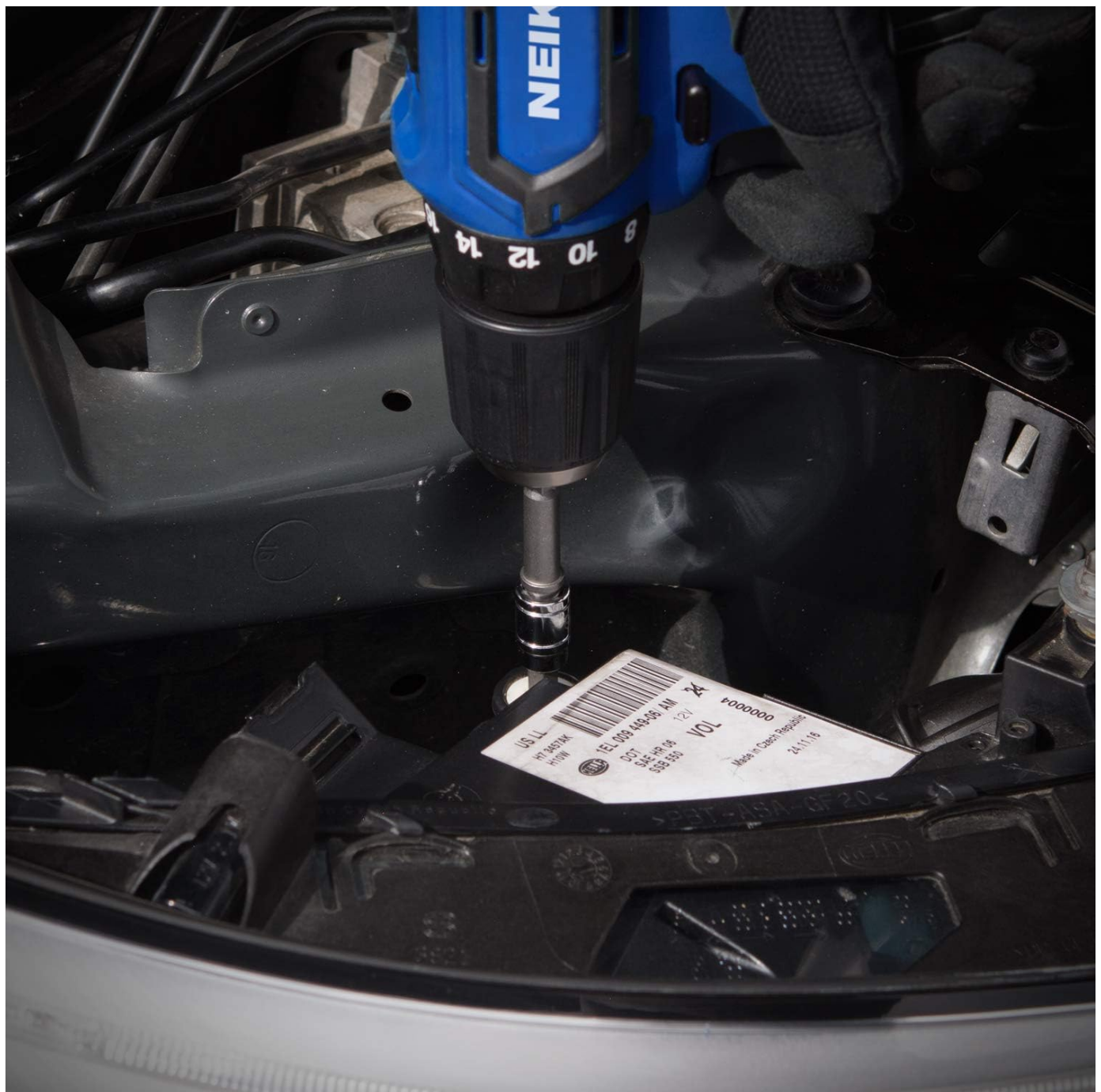
Figure 4: The socket adapter being used in an automotive repair scenario, illustrating its practical application in tight spaces and for various mechanical tasks.
