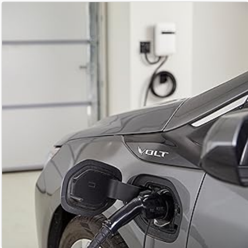
Image 6: A detailed view of an electric vehicle's charging port with the J1772 connector securely inserted, indicating an active charging connection.
