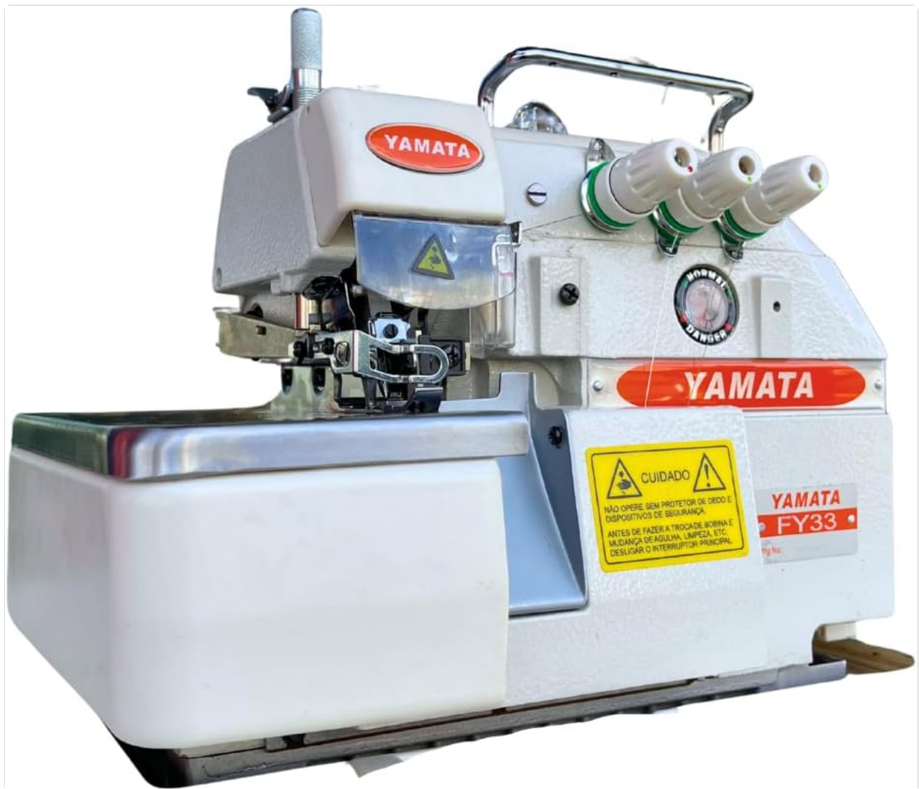
Frontal view of the YAMATA FY33 overlock machine head, highlighting safety warnings and critical areas.
