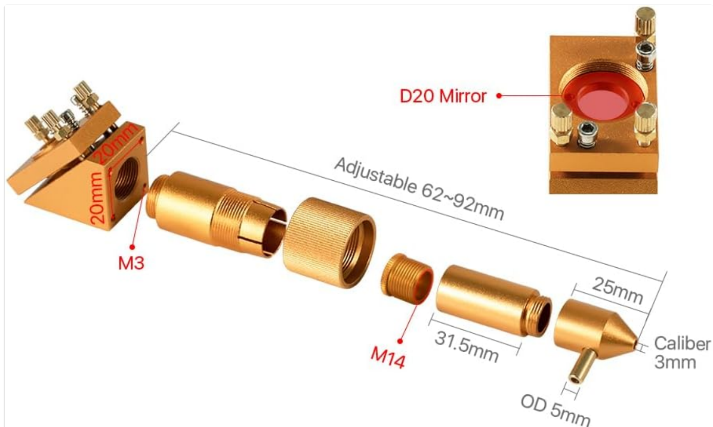
Figure 3.1.1: Exploded view of the laser head, showing adjustable length (62-92mm) and M14 thread for lens tube. Caliber 3mm, OD 5mm.
