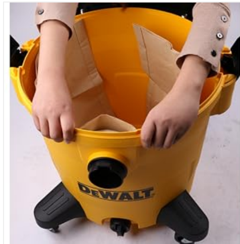
Figure 3: Example of a dust bag installed within a shop vacuum.
