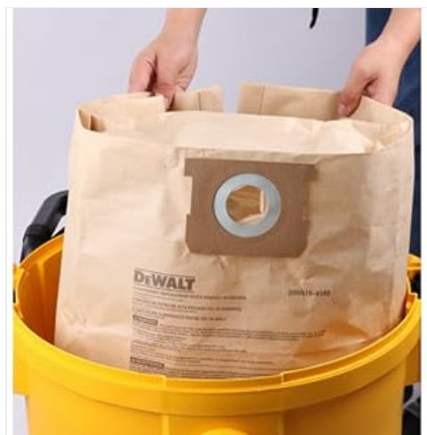
Figure 5: Removing a dust bag from the vacuum tank.
