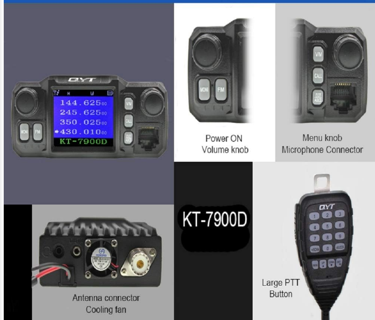
Figure 3.1: Front and rear views of the KT-7900D radio and its microphone, highlighting key features.
