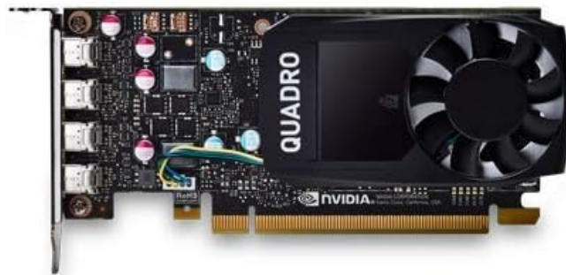
Side view illustrating the cooling fan and low-profile bracket.
