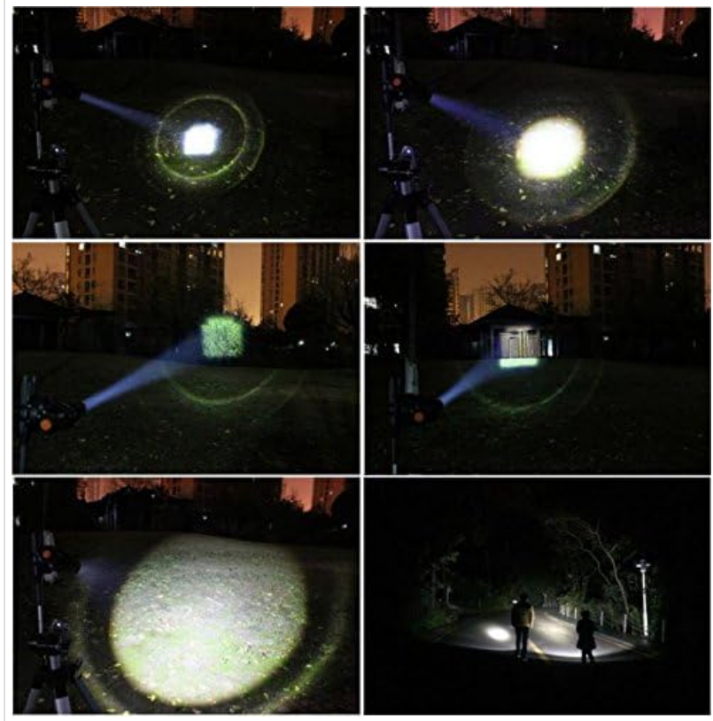
Figure 6: Various beam patterns demonstrating the effect of the zoom function in different environments.
