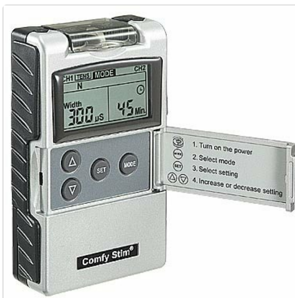
Figure 1: Front view of the Biotronix Comfy Stim EV-806 with the protective cover open, displaying controls and basic instructions.
