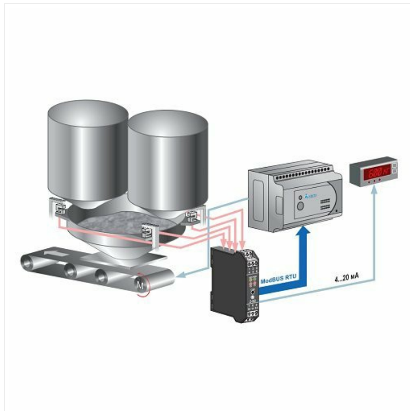
Figure 4: Example application diagram demonstrating the Z-SG module integrated into a weighing system, connecting load cells to a control unit via Modbus RTU and providing an analog output to a display.
