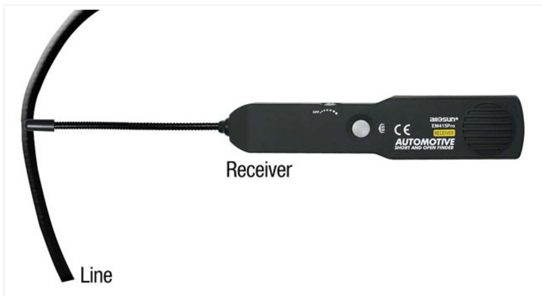
Figure 4: Proper positioning of the receiver probe for optimal signal detection.
