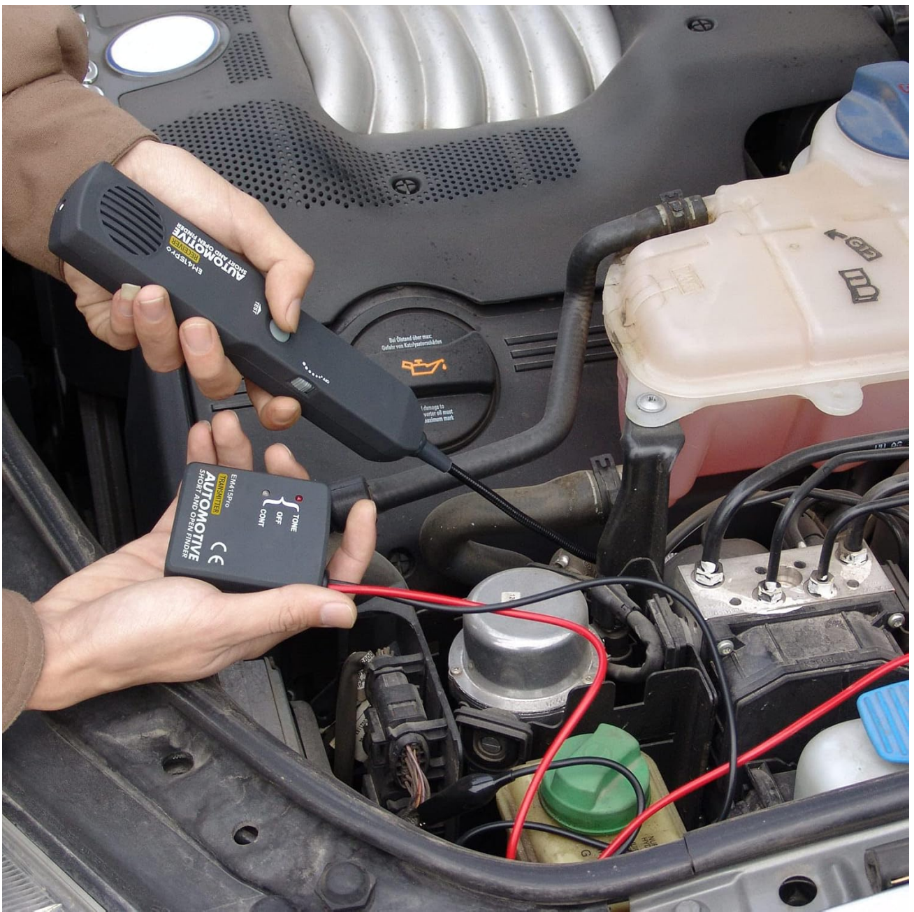
Figure 5: Using the EM415Pro to diagnose electrical issues in an automotive engine compartment.
