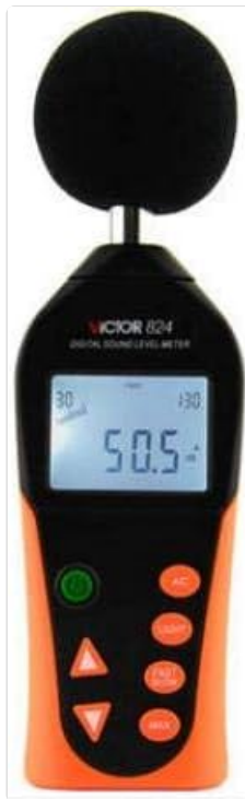
Figure 1: Front view of the Victor 824 Digital Sound Level Meter, showing the display and microphone.
