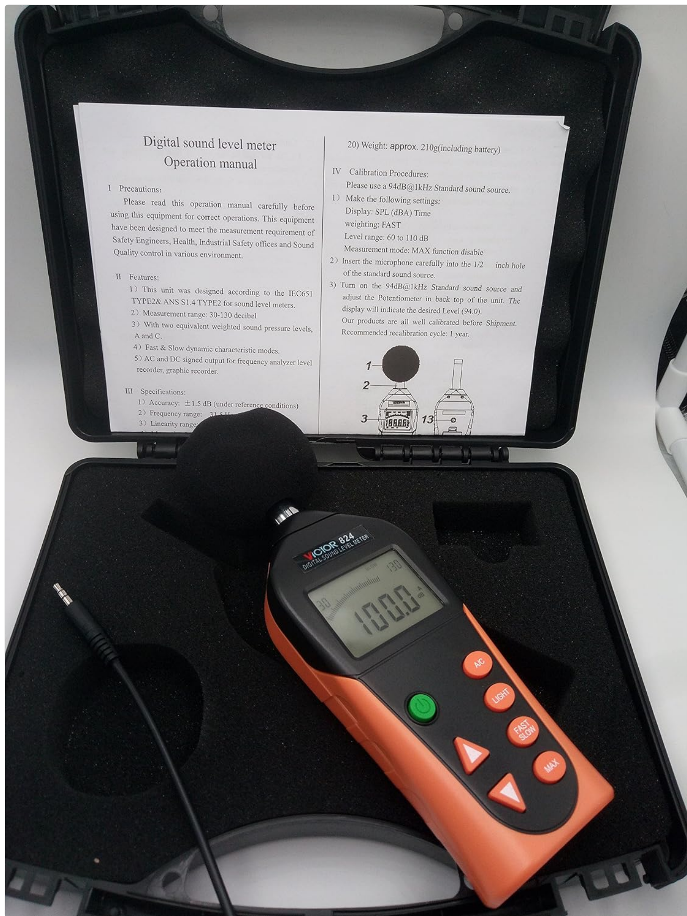
Figure 4: The Victor 824 Sound Level Meter stored in its protective carrying case.
