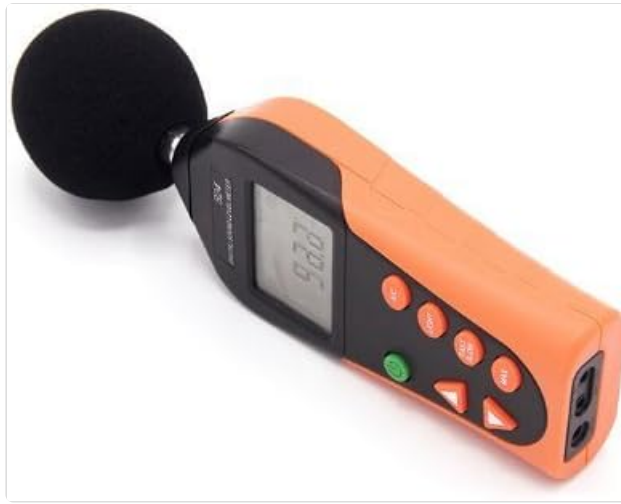
Figure 3: Side view of the Victor 824, illustrating the AC/DC output ports.
