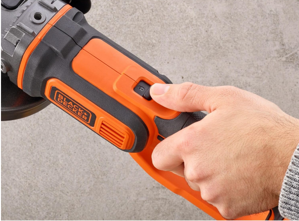
Figure 5.1: Engaging the on/off switch for tool operation.
