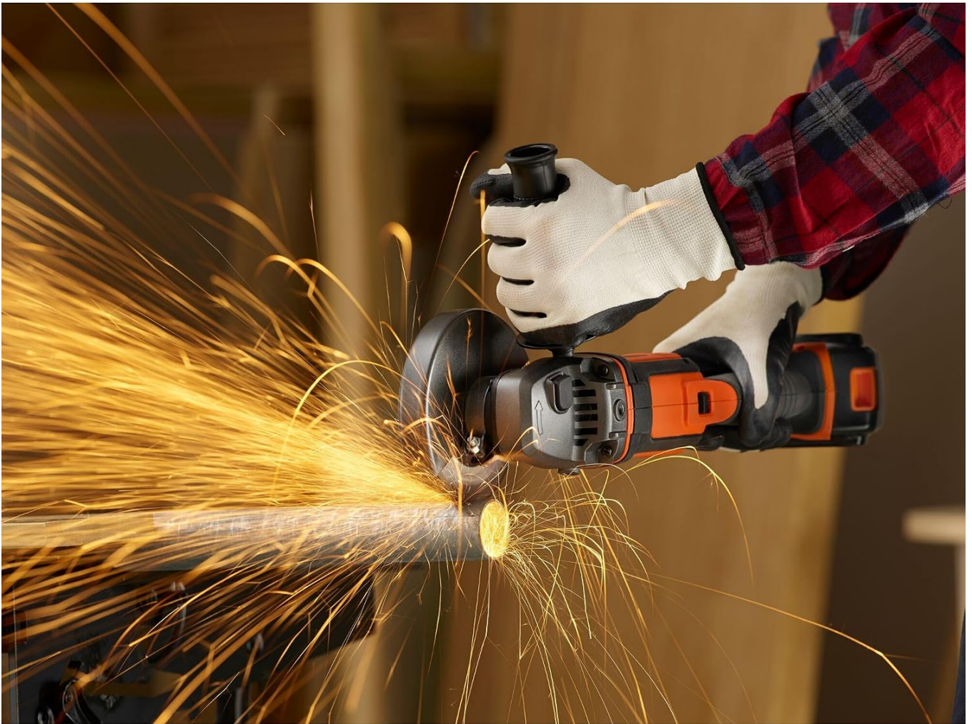
Figure 5.3: Demonstrating metal cutting with the angle grinder, showing sparks generated during operation.
