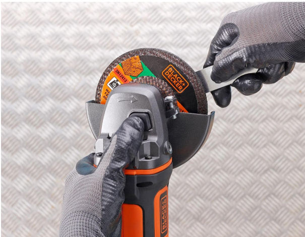
Figure 4.2: Using the provided tool to secure or remove the grinding/cutting disc.
