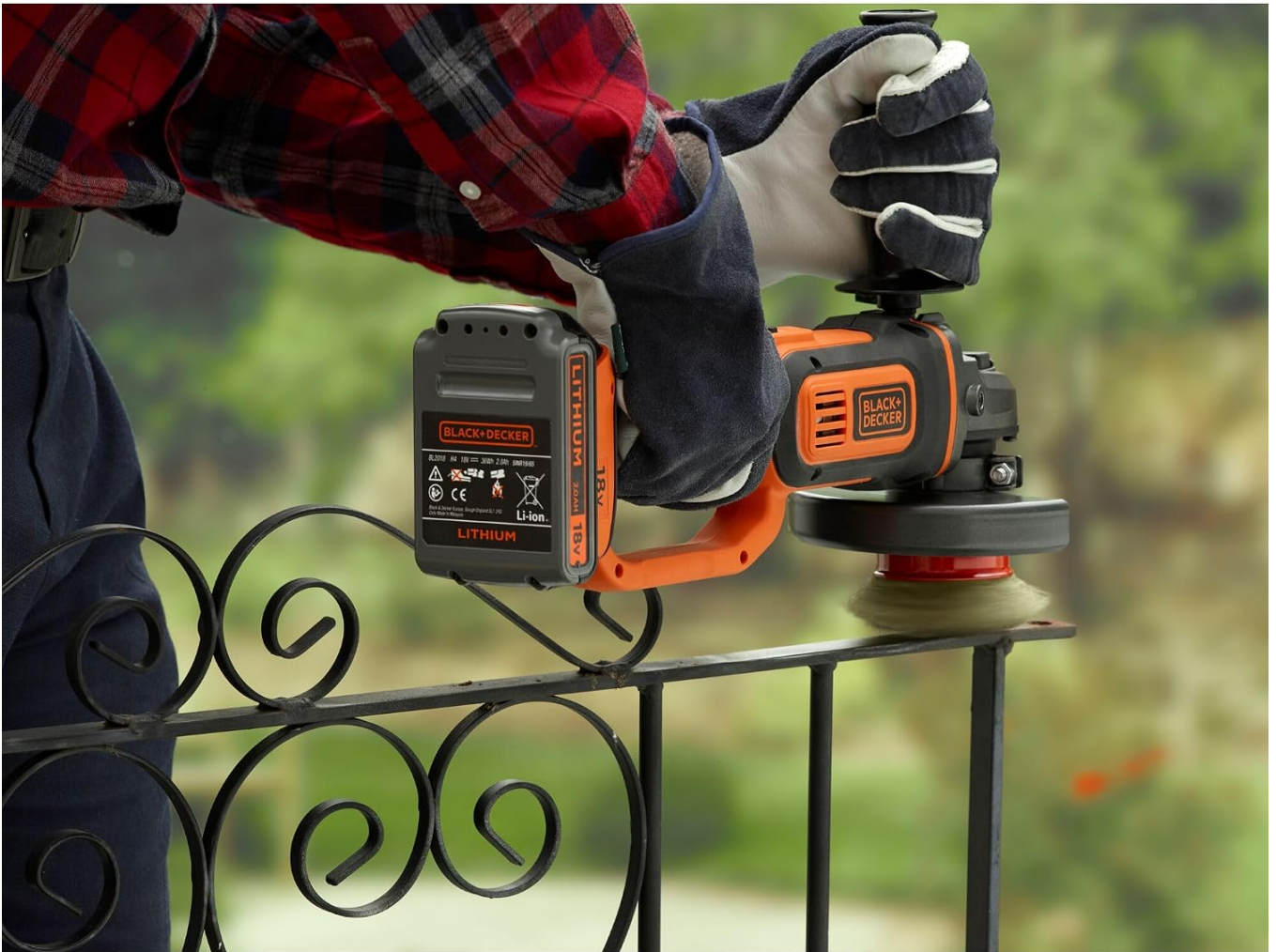
Figure 5.4: Using a wire brush attachment on the angle grinder to clean or prepare a metal fence surface.
