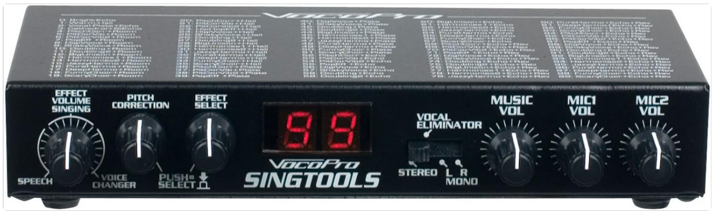
Figure 4.1: Front Panel Controls of the VocoPro SINGTOOLS Mixer. This image displays the various knobs and the digital display, including controls for Effect Volume, Pitch Correction, Effect Select, Vocal Eliminator, Music Volume, and Microphone Volumes.
