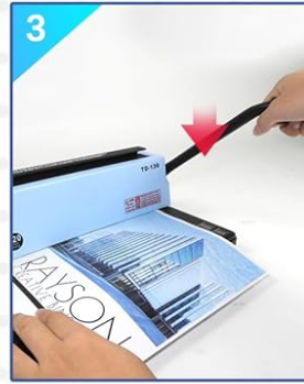
3 Secure the documents and press the lever to punch holes
