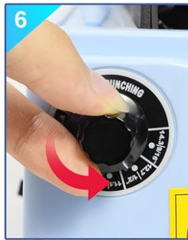
6 Adjust the knob to the wire size
