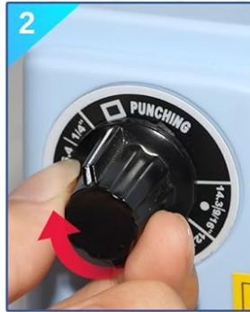
2 Turn the knob to the "Punch" position
