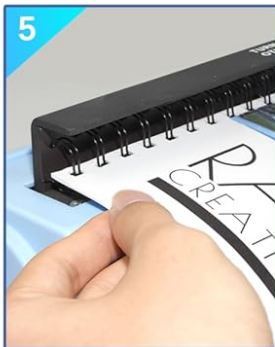
5 Position the wire and documents in the binding plate
