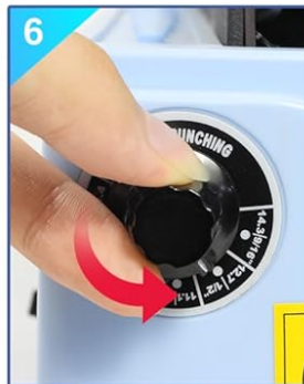
6 Adjust the knob to the wire size
