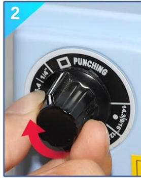
2 Turn the knob to the "Punch" position
