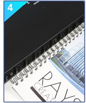
4 Place the punched documents onto the wire
