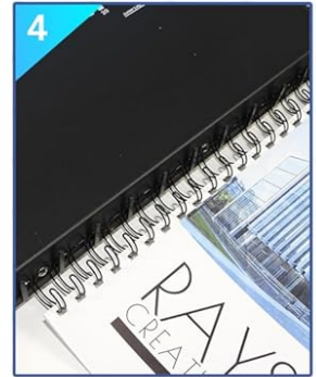
4 Place the punched documents onto the wire
