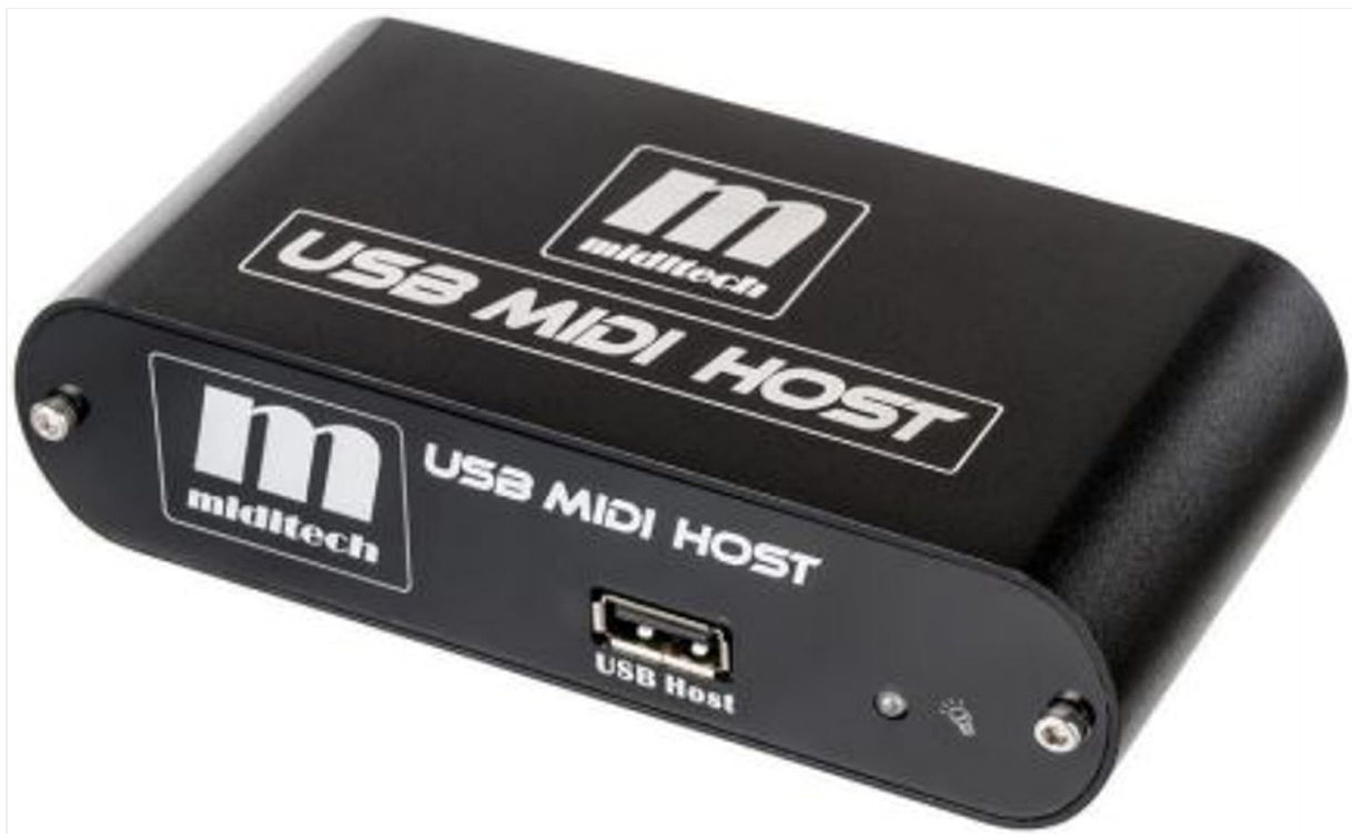
Figure 1: Front View of the Miditech USB MIDI Host. This image shows the front of the device, highlighting the USB Host port (Type A) where your USB MIDI controller connects. The Miditech logo and "USB MIDI HOST" text are clearly visible.
