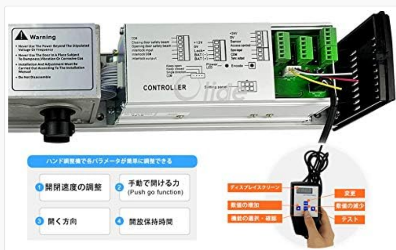
Figure 3.2: The controller unit with its various terminals for connections and a handheld programmer for parameter adjustments. The programmer allows for setting opening speed, manual push function, opening direction, and hold-open time.
