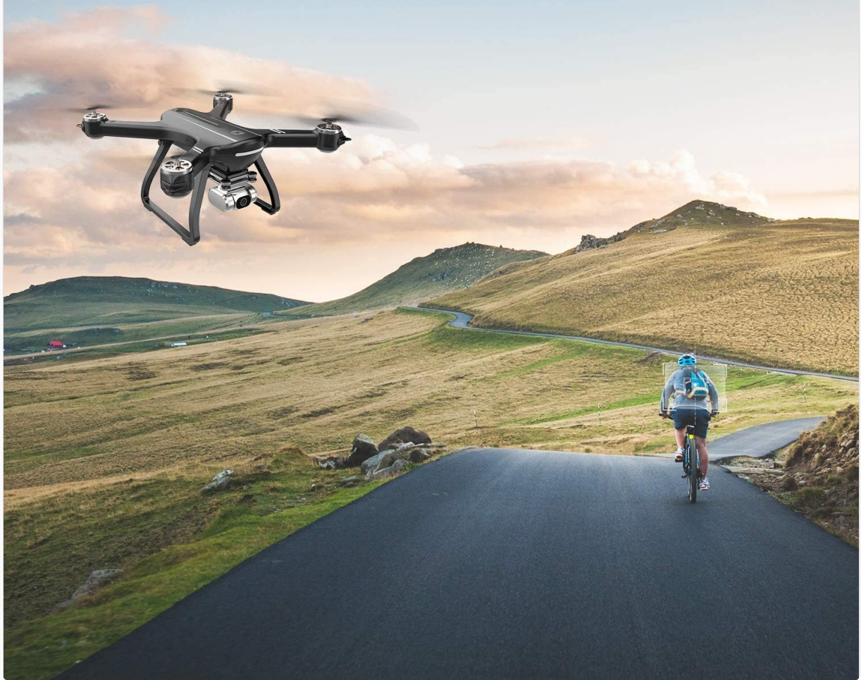
Figure 4.2: Holy Stone HS700D drone operating in Follow Me Mode.
