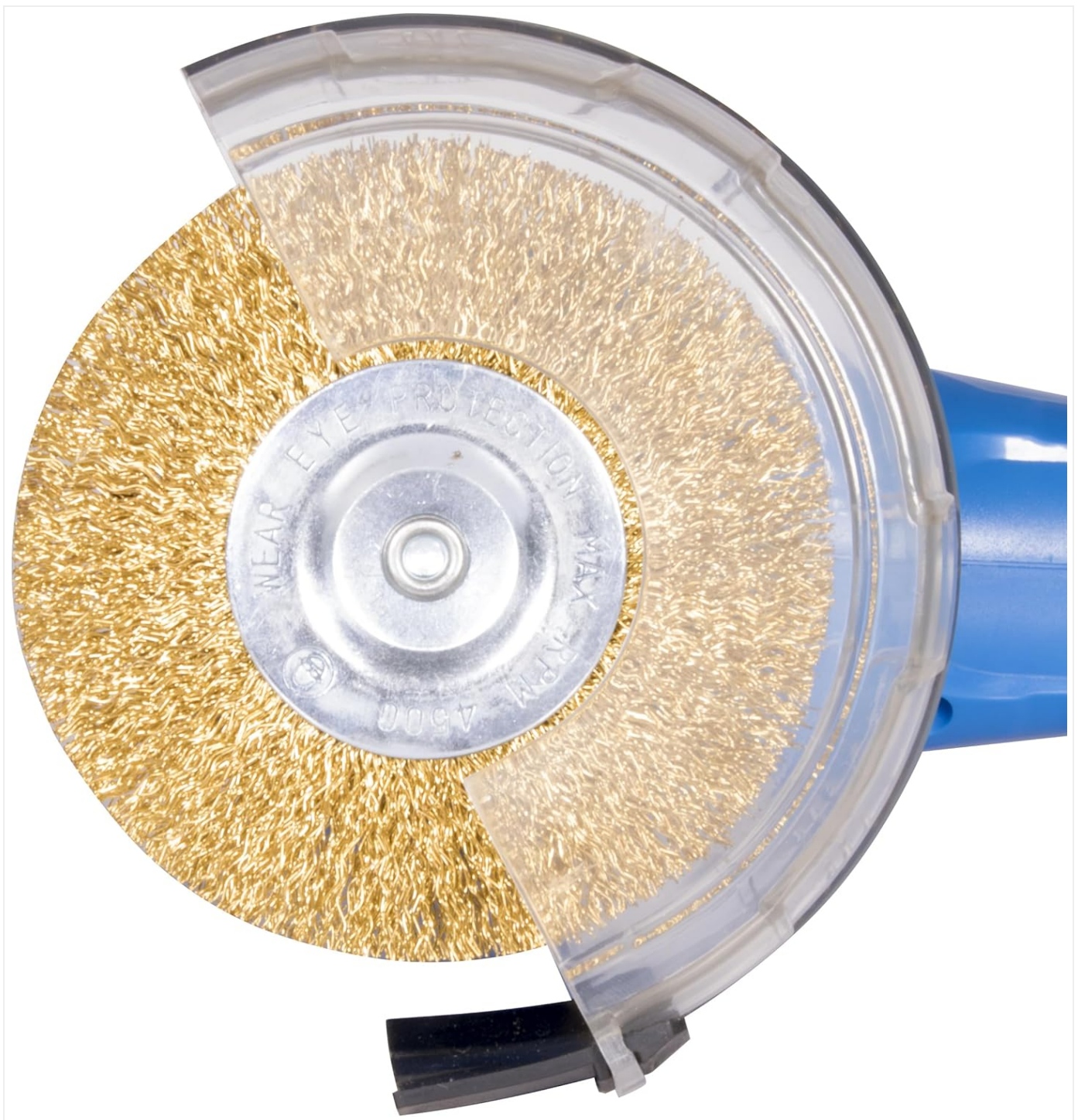
Figure 4.2.2: Metal brush installed.
