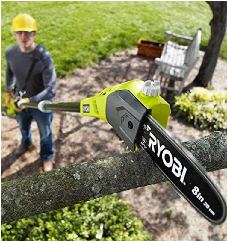
Image 4: An individual demonstrating the use of the Ryobi ONE+ pole saw to trim an overhead tree branch.
