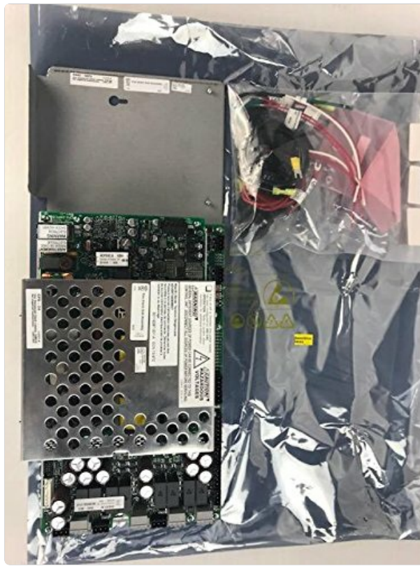
Figure 2: The Notifier DAA2-5025 Digital Amplifier along with its accessory components, as typically received in its packaging. This image provides a view of the complete product and included parts before installation.
