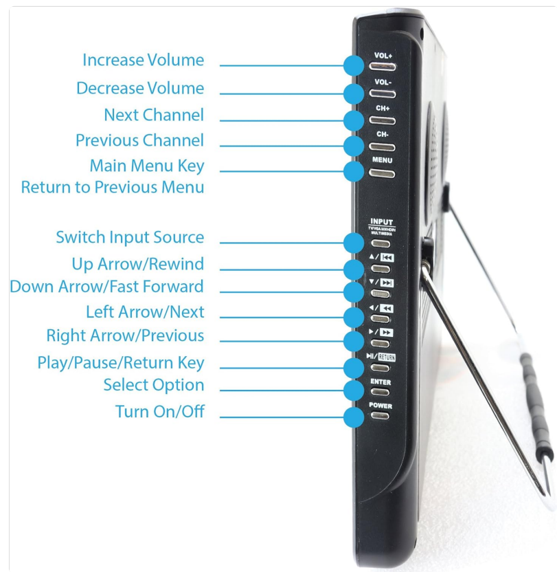
Figure 2: Side panel controls. These buttons allow for direct control of the TV's functions without the remote.
