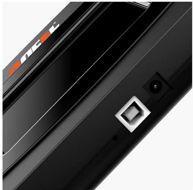
Image: Detailed views of the ANCEL FX4000's diagnostic port, USB port, and screen interface.
