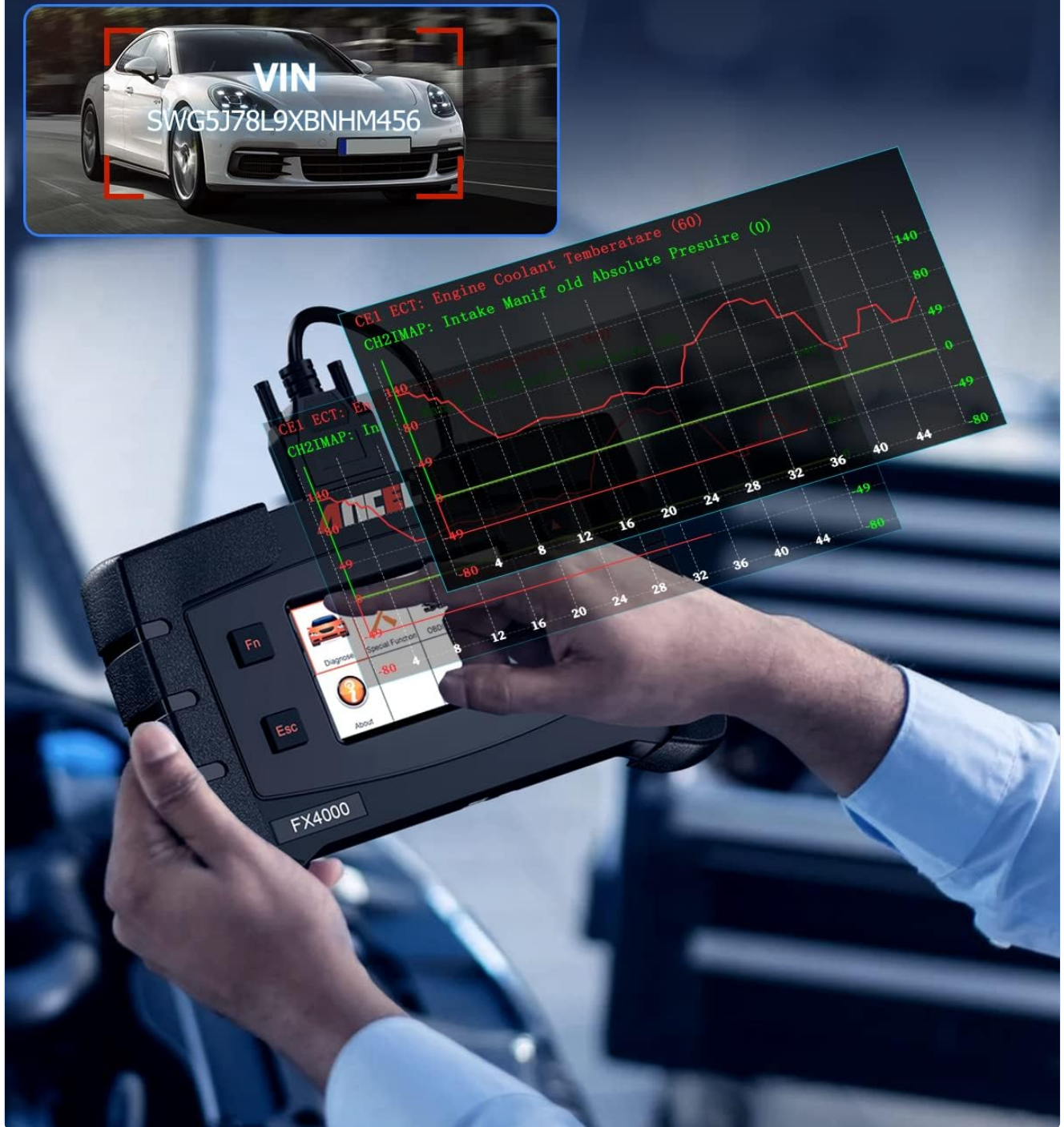
Image: The ANCEL FX4000 showing a live data stream graph and an automatic VIN scan feature.
