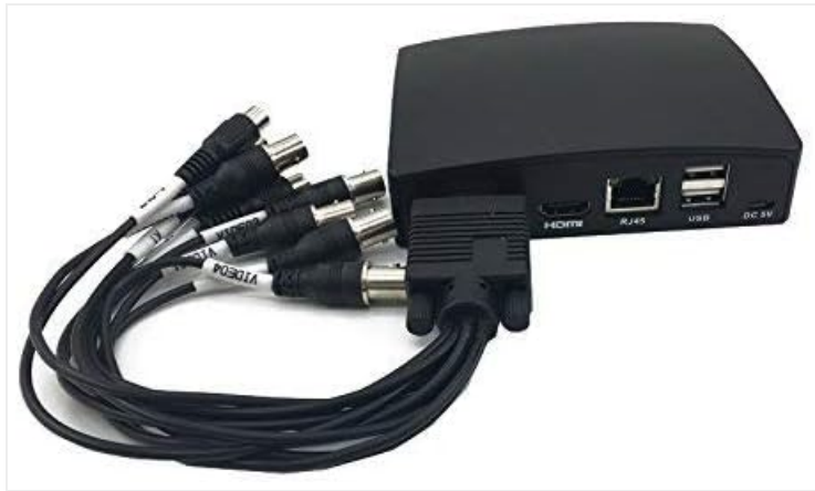
Figure 4.2.1: DVR with BNC cable connected for camera inputs.
