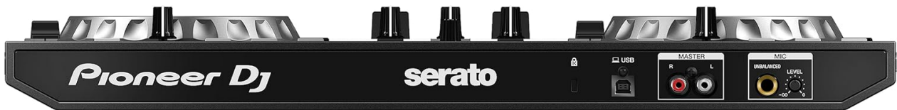
Figure 2: Rear view of the DDJ-SB3, showing USB, Master RCA outputs, and Microphone input.
