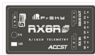
Image 3: Detailed diagram of the FrSky RX8R PRO receiver, illustrating the F/S button, LED, Smart Port, SBUS OUT, SBUS IN, and 8 PWM channel outputs.
