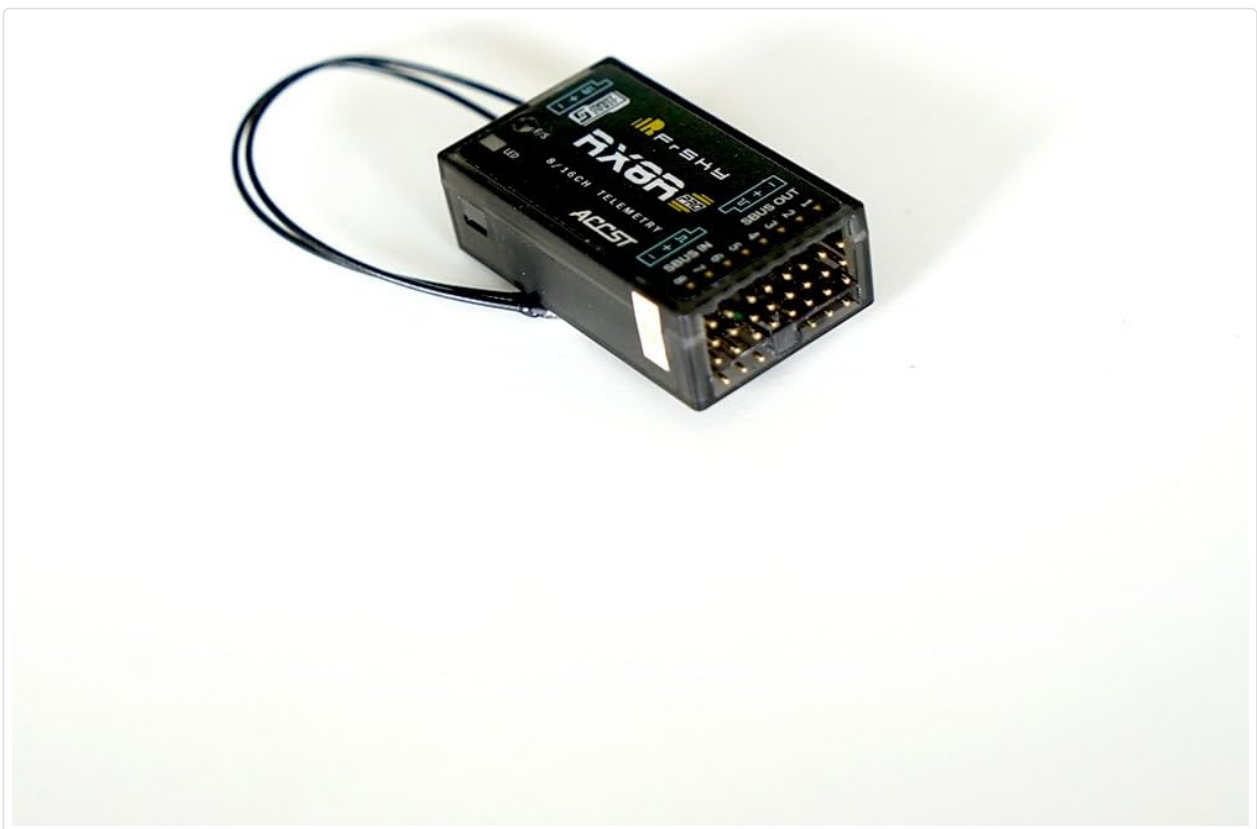
Image 2: Angled view of the FrSky RX8R PRO receiver, highlighting the servo pin headers and antenna connections.
