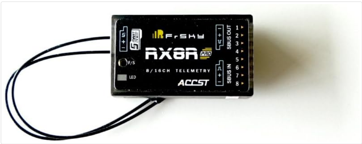
Image 1: Top view of the FrSky RX8R PRO receiver, showing the F/S button, LED indicator, Smart Port, and servo/SBUS output pins.
