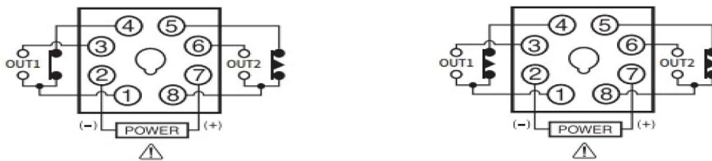
Figure 4: Detailed specifications of the T48A timer (top) and connection diagrams for T48A-B and T48A-C models (bottom).
