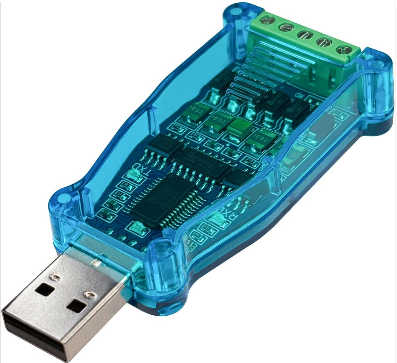
Image: The DSD TECH SH-U11 USB to RS485 RS422 Converter, a compact device with a transparent blue casing, USB-A connector, and a 5-pin terminal block.
