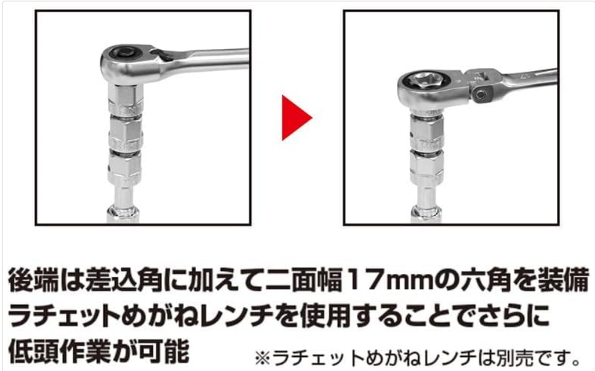
Image 4: Illustration demonstrating how a 17mm ratchet glasses wrench can be used on the outer hexagonal part of the extension bar for initial loosening or final tightening in extremely low-clearance situations.
