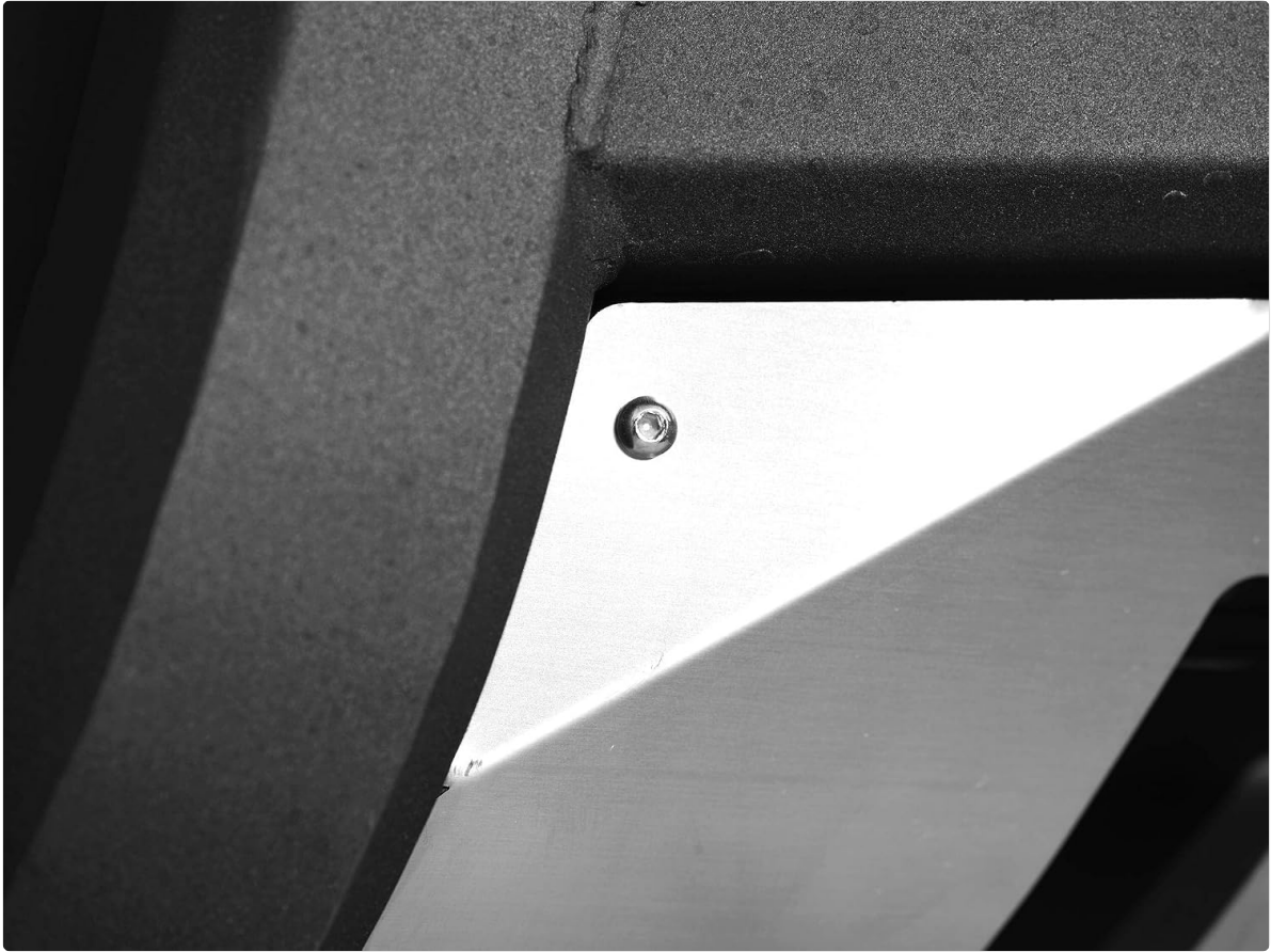
Figure 3: Detail of a bolt securing the skid plate component.
