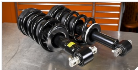
Image 5.1: Example of a complete coilover assembly, similar to the components in the conversion kit.
