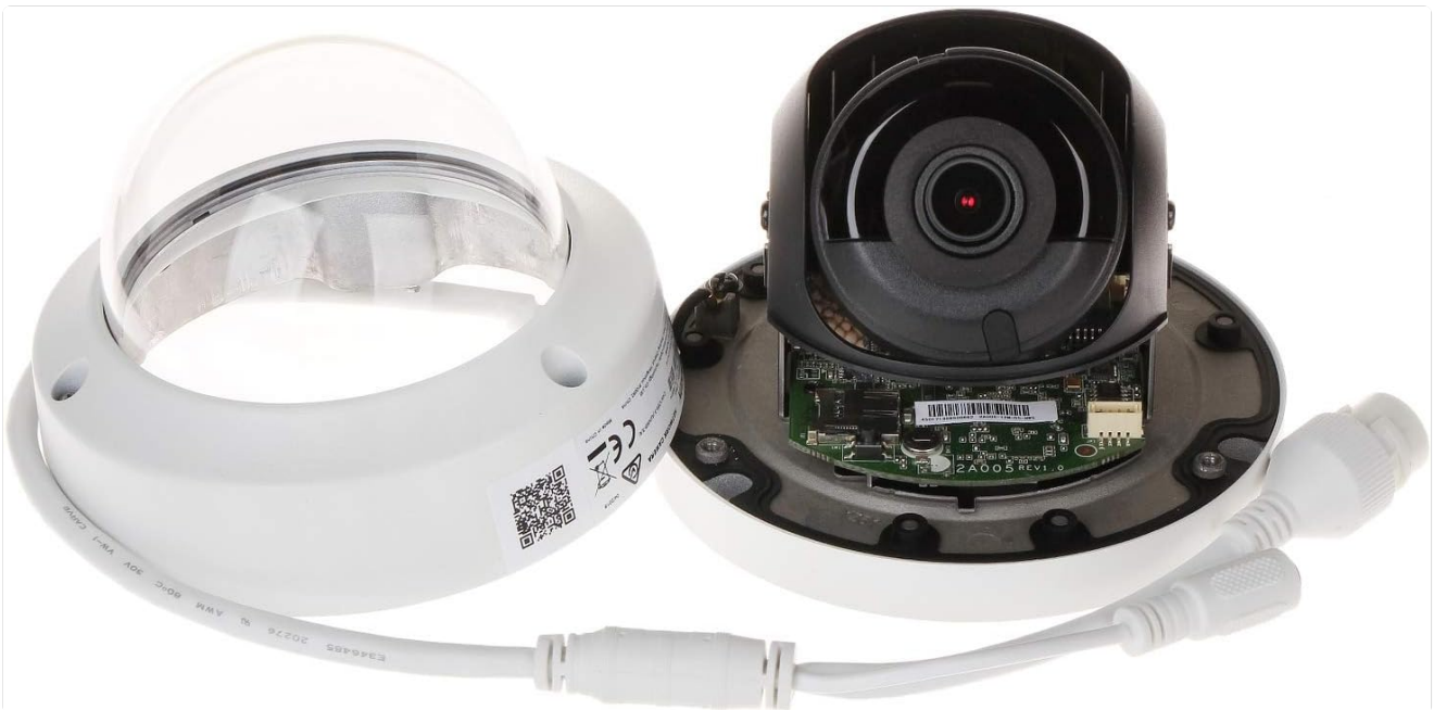
Figure 4.2: Internal view of the camera with the dome cover removed, revealing the camera module and base plate.
