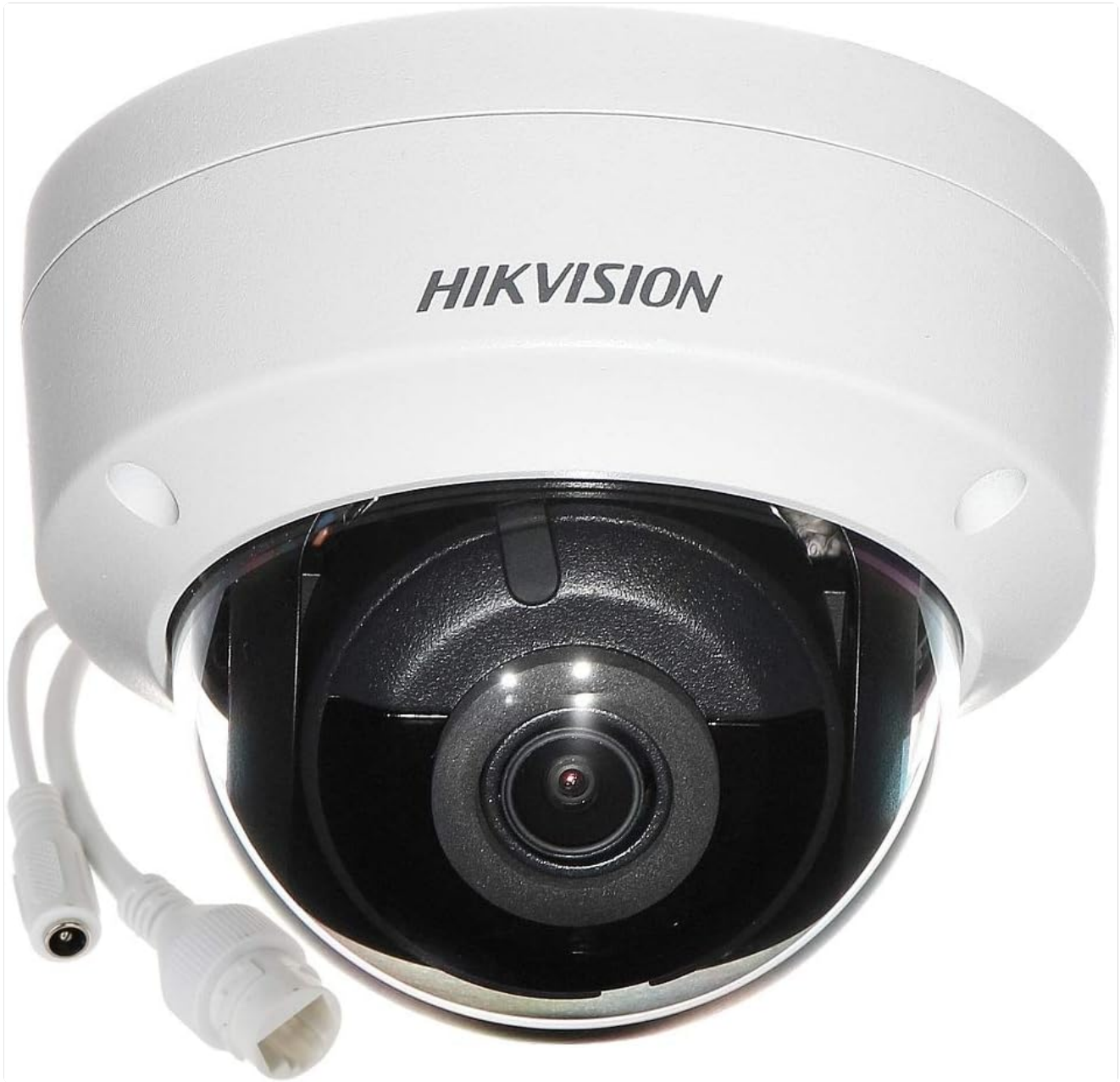
Figure 4.1: Front view of the Hikvision DS-2CD2143G0-I camera, showing the dome housing and lens.
