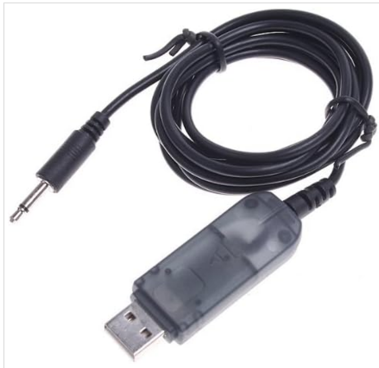
Image 3.2: The main USB simulator cable, which connects to the computer.
