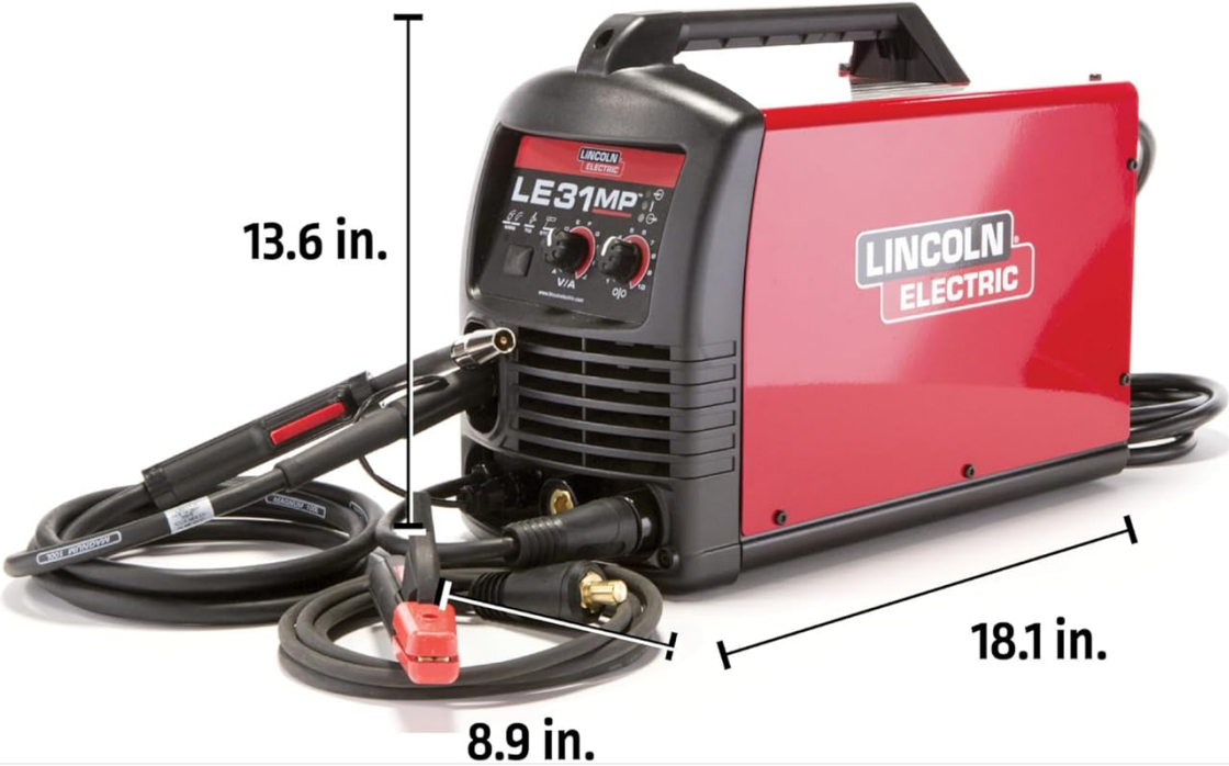
Figure 8.1: Physical dimensions of the LE31MP welder unit.
