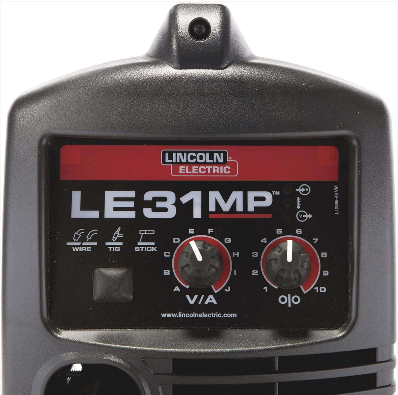
Figure 5.1: Detailed view of the LE31MP control panel. The left knob adjusts voltage/amperage, the right knob adjusts wire feed speed, and the switch selects the welding process.
