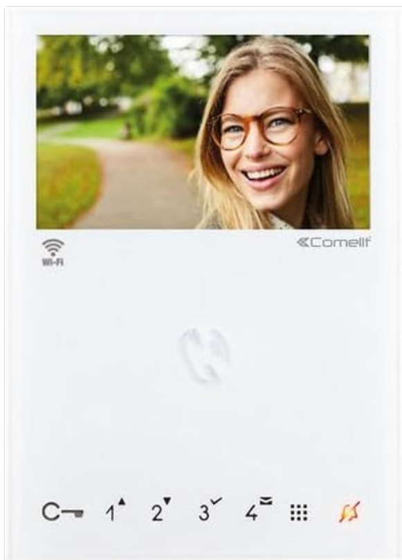
Figure 1: Front view of the Comelit 6741W Monitor Mini, showing the display and control buttons.
