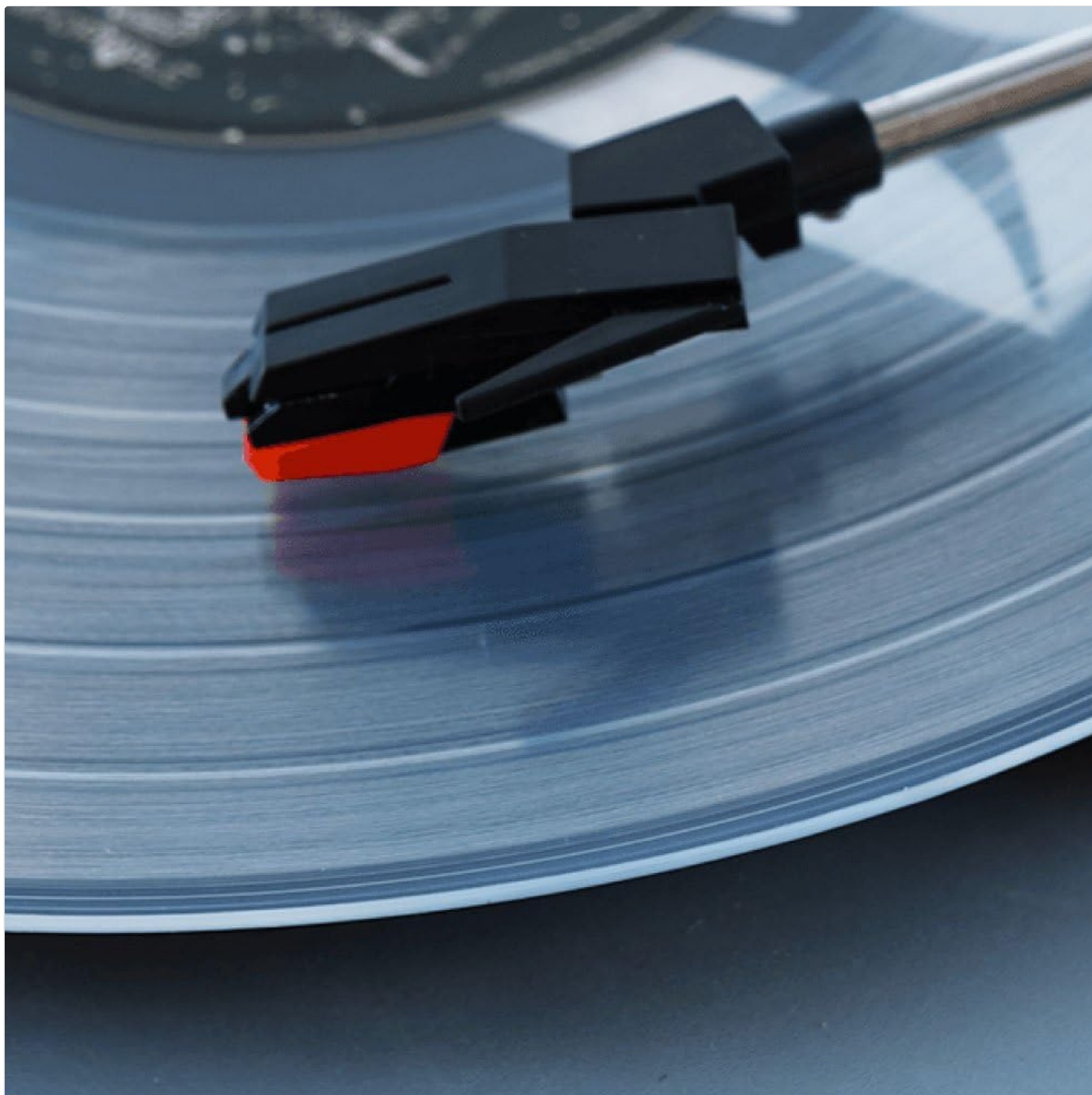
Image: A close-up shot of the turntable's stylus cartridge resting on the grooves of a vinyl record.
