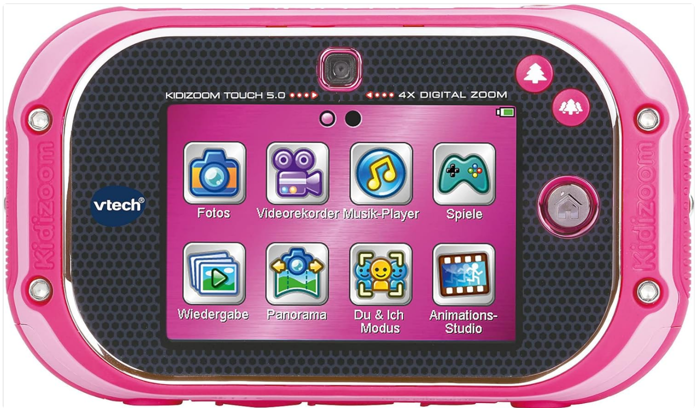
Figure 3: The camera's 3.5-inch LCD color touch display showing the main menu with icons for photos, video recorder, music player, games, playback, panorama, 'You and Me' mode, and animation studio.
