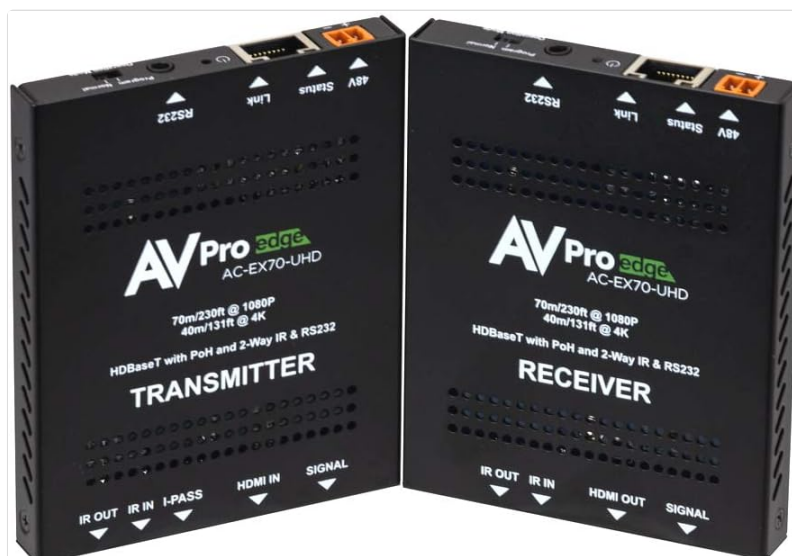
Image: The AVPro Edge AC-EX70-UHD Transmitter (left) and Receiver (right) units, showing their labels and port layouts.
