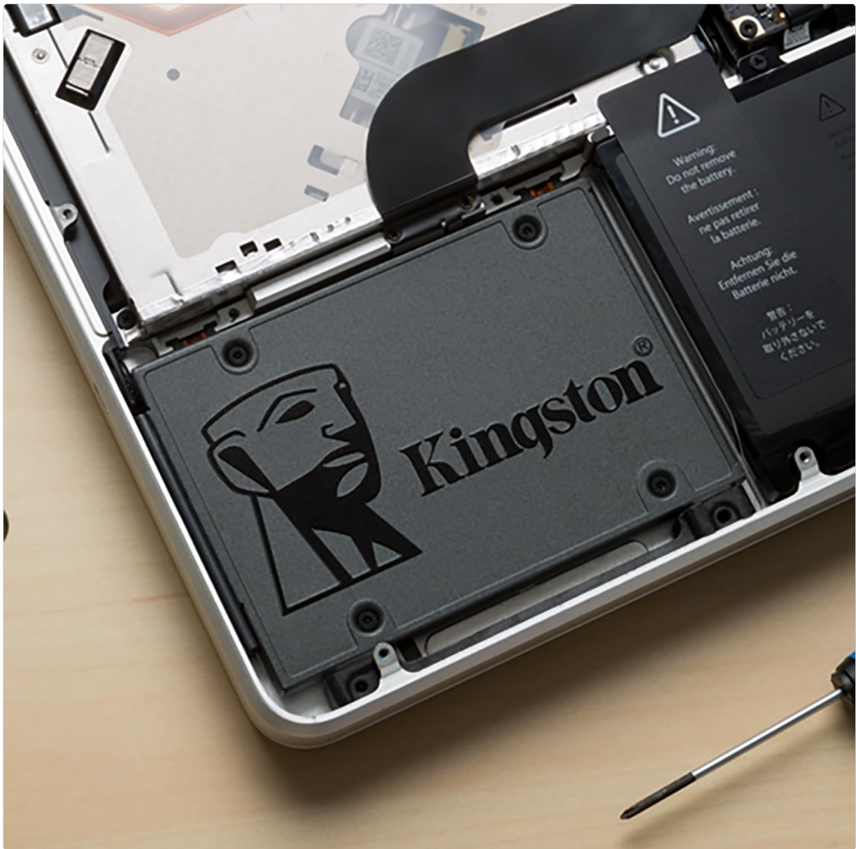
Figure 5: The Kingston A400 SSD fully installed within a notebook computer's drive bay.
