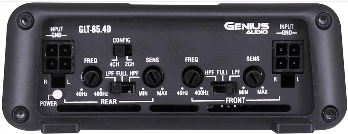
This image displays the input side of the GLT-85.4D amplifier, detailing the various controls and connections. It includes RCA input terminals (R, L) for both Rear and Front channels, gain controls (SENS MIN/MAX), frequency adjustment knobs (FREQ 40Hz-400Hz), and crossover switches (LPF, FULL, HPF) for both Rear and Front channels. A configuration switch (CONFIG 4CH, 2CH) is also visible, along with the Power indicator light.
